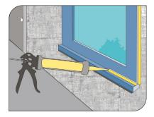
**Tekadom Acryl Woodenwood** is a one-component extremly flexible plastoelastic sealant based on special acrylic dispersion.
